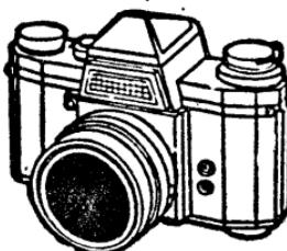
Praktica IVB with built-in exposure meter. The IVM and IVF models were also fitted with exposure meters as IVBM and IVFB.
