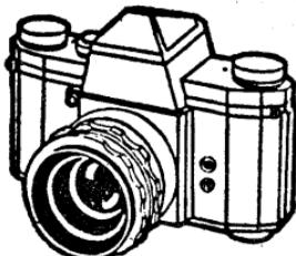
Praktica FX2 permitted the attachment of a pentaprism and had semi-automatic aperture setting. Later versions had fully automatic iris control.
