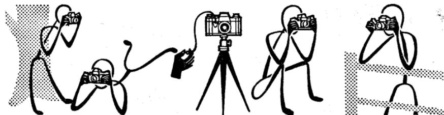
Above: With the Praktica it is specially important to keep the camera really steady during the exposure and for a fraction of a second after pressing the release button. Whenever possible support your body against something solid, such as a tree or wall or prop up your hands against your knees or a table, particularly with slow speeds. Use a cable release for time exposures from a tripod (page 12).
