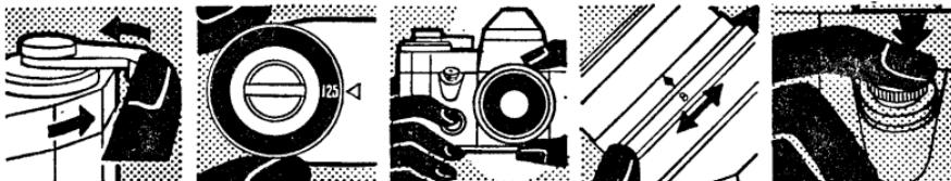
Shooting with the Praktica Nova. From left to right: Transport film and tension shutter with the rapid wind lever; set the shutter speed; focus the image on the screen; pre-select the aperture; press the shutter release smoothly and gently.
